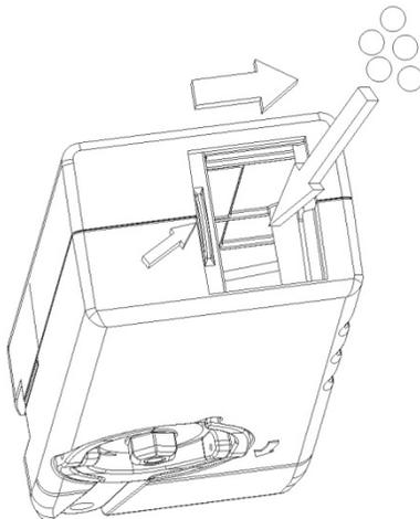
Load BBs into the BB reservoir. Once the BB reservoir is full, slide the door closed.
