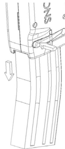
Depress the magazine release latch, and remove the magazine. Repeat steps 1-6 to load additional magazines
