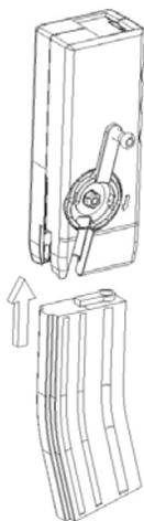
Insert your magazine into the bottom of the M12 sidewinder. The magazine should audibly "click" into place.
