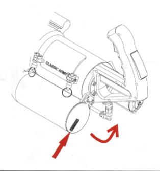
Insert the gas bottle to the botton and tight clockwise quickly.
