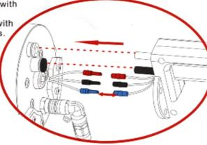
3. Connected wires and tubes and push grip to fit body. aim to 4 screw holes and tight 4 scerws M5\*12 by scerw driver.
