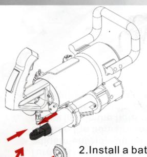
Install a battery to battery storage and close the cap.
