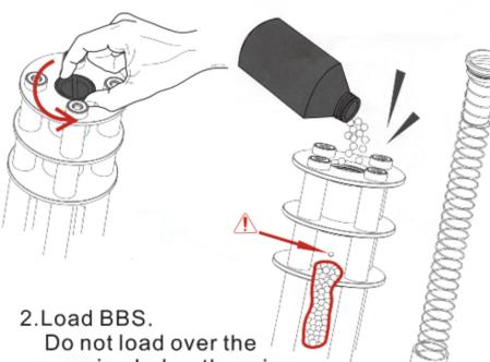
Press the spring into the tube and insert it, into the slot and tight it clockwise.
