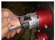
After thunder core is ready, remove the simulator bomb safety pin and use it to load the thunder grenade hammer .
