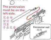
Store the battery in the receiver as shown. (Set the battery so that it does not protrude.)
