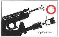
Make sure to attach the protective plug to the gun muzzle, except when you are shooting, for preventing accidental, sudden discharge and for the dust-proof purpose. (Never pull the trigger with the protective plug being attached.)
